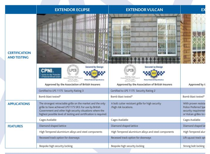
BOMB BLAST MITIGATION\*: In bomb blast mitigation tests the Eclipse and Vulcan grilles were successfully tested in conjunction with glass backed with anti-shatter security film usi
